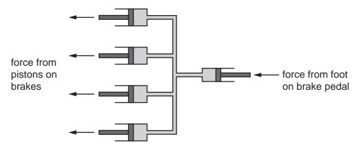
The pipes are filled with incompressible liquid. When a force is applied to the brake pedal, the pressure in the liquid increases and applies a force to each of the four wheels.
